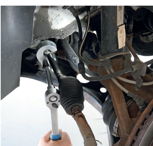
📷 3: Releasing / tightening the inner track rod.
