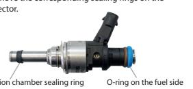
**© 2:** Pre-stretch the combustion chamber sealing ring.
