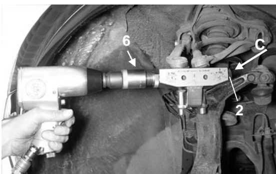
Fig. 3: Retaining bolt removal (pressure drift I).
