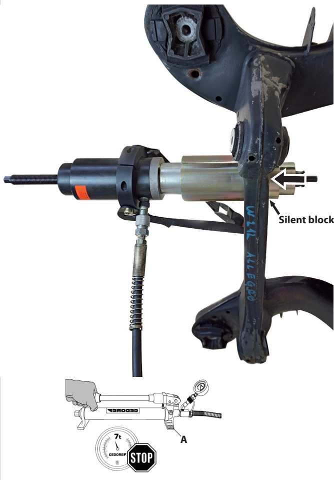
Fig. 12: Pull silent block C from the rear axle beam.
