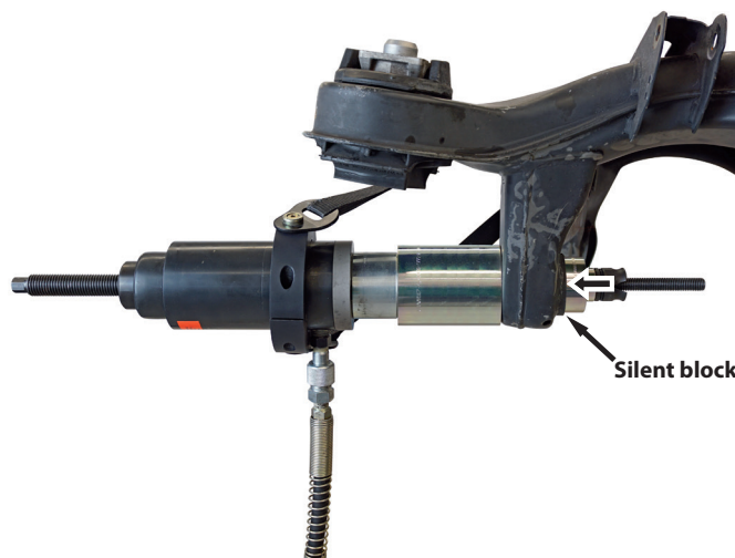
Fig. 18: Pull the silent block D on the rear axle beam.
