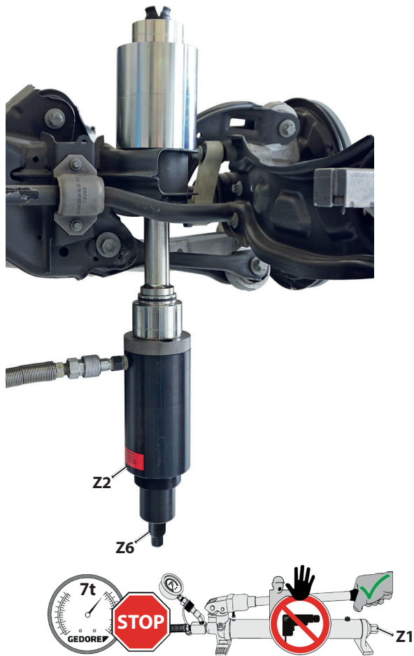
📸10: Applying the silent block tool to the rear axle carrier.
