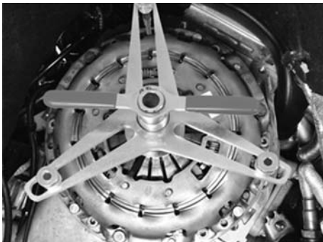
Fig. 3: Pretensioning and installing the clutch pressure plate with KL-0500-45
