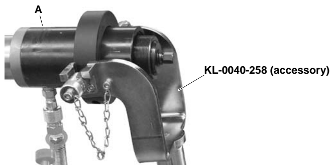
Fig. 3: Mounting the hydraulic cylinder into retaining device.
