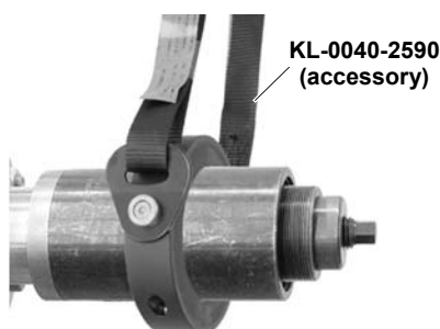
Fig. 4: Fixing the safety belt to hydraulic cylinder.
