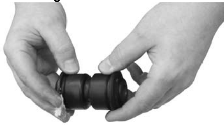
Fig. 7: Lubricating the silentbloc.
