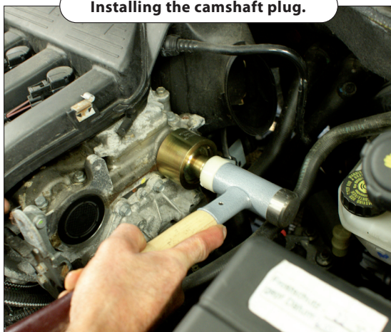
Installing the camshaft plug.
