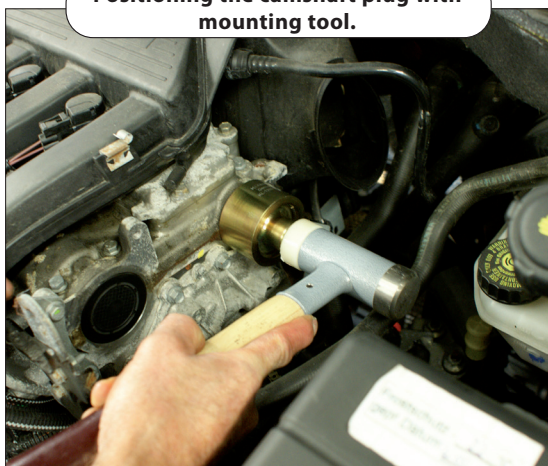
Positioning the camshaft plug with mounting tool.
