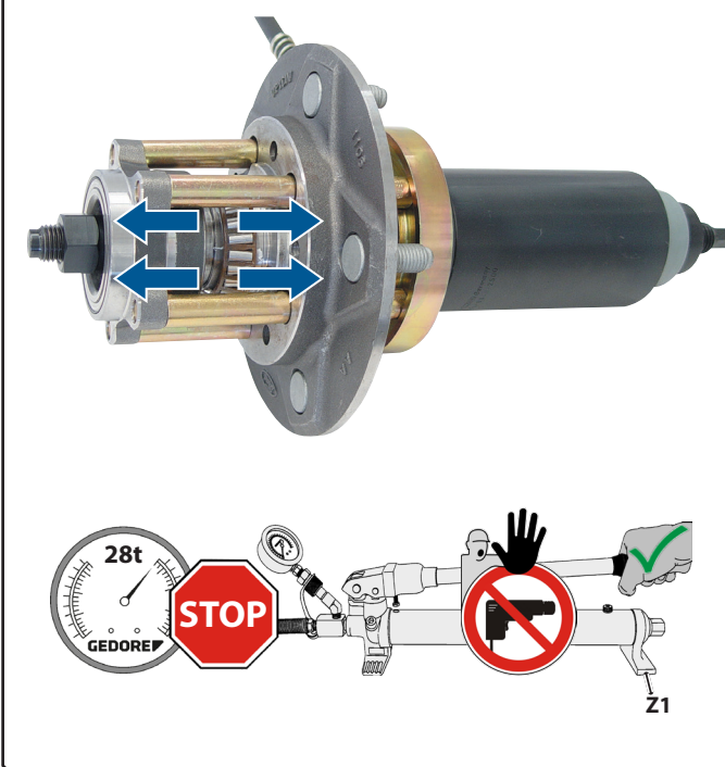
📷 12: Forcing the wheel hub out of the wheel bearing unit.
