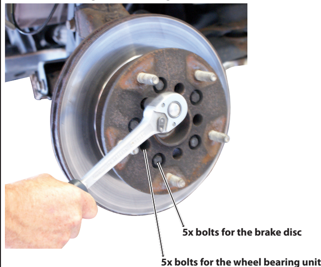
📷3: Unscrewing the fastening screws.
