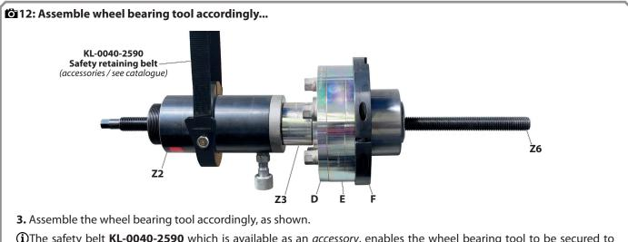
(i) The safety belt KL-0040-2590 which is available as an accessory, enables the wheel bearing tool to be secured to prevent it from falling down or flinging around.
