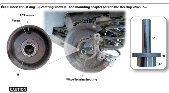
The ABS sensor can be damaged when pressing in the wheel bearing unit!
