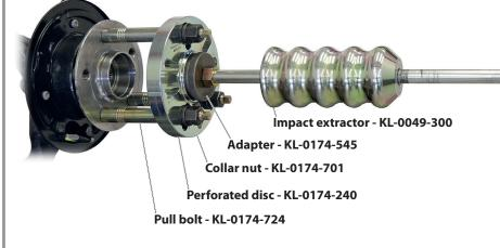
1A. Pull out the wheel hub as shown, using the KL-0174-.. Puller series available as an accessory. Always follow the corresponding instructions.
