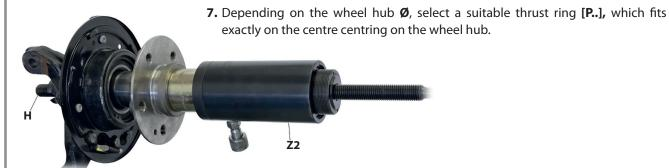
8. Prepare the hydraulic cylinder [Z2] accordingly as shown and insert it with the **PULL SIDE** on the wheel bearing.
