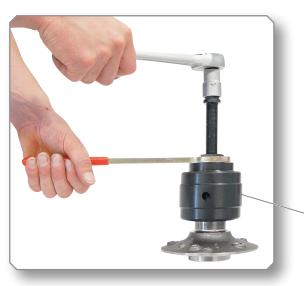
(i) If the wheel hub is to be used again, the wheel bearing inner ring must be removed first. For example, with the help of the **puller kit for bearing inner rings - KL-0042-90 K**, which is available as an *accessory*
