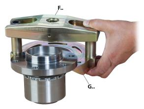
**1.** Place the bridge **[F..]** with the tension/pressure plate **[G..]** in the correct position on the new wheel bearing unit as shown.
