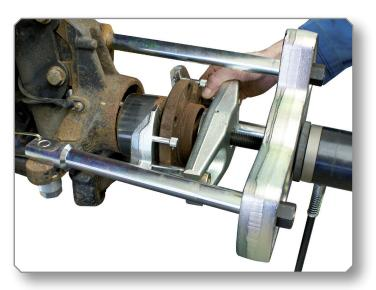
**14.** Remove the wheel bearing unit with bridge **[F..]** and tension/pressure plate **[G..]**. and clean the wheel bearing bore on the steering knuckle.
