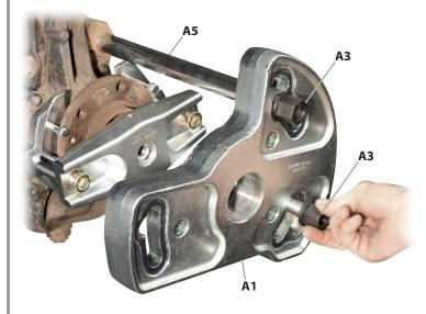
**7.** Place the base plate [A1] in the correct position on the support rods [A5] according to the **hole distance** of the base strip [E...] as shown.
