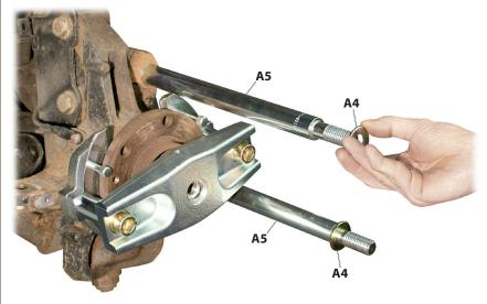
**6.** Place one washer **[A4]** on each of the support rods **[A5]**.
