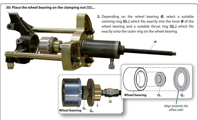
**3.** Place the mounting adapter **[L]** together with the matching centring ring **[O..]**, thrust ring **[Q..]** and wheel bearing in the correct position on the clamping nut **[I2]** as shown. Then screw in the pull spindle **[H]** until the
