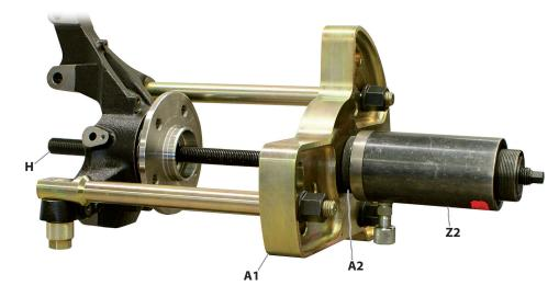
7. Prepare the hydraulic cylinder [Z2] accordingly as shown and subsequently screw it in with the PULL SIDE to the base plate [A1].
