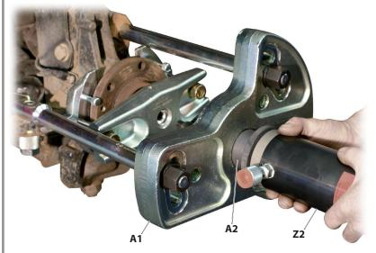
**11.** Prepare the hydraulic cylinder **[Z2]** accordingly as shown and subsequently screw it in with the **PULL SIDE** to the base plate **[A1]**.
