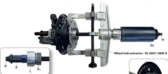
1B. Pull out the wheel hub as shown using the KL-0041-380 A - Wheel hub
