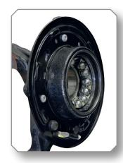
©36: Pull out the wheel hub, for example, using the KL-0041-380 A - Wheel hub extractor (accessory)...
