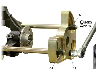
**5.** Tighten the <u>three</u> collar nuts **[A3]** uniformly to **25Nm**.
