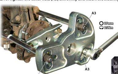
**9.** Tighten the three collar nuts [A3] uniformly to 25Nm.
