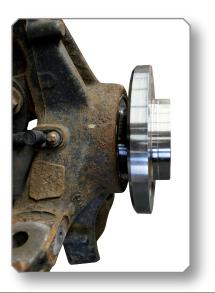
**8.** Check the correct installation position of the wheel bearing unit, remove the wheel bearing tool and reassemble the vehicle according to the <u>manufacturer's specifications</u>.
