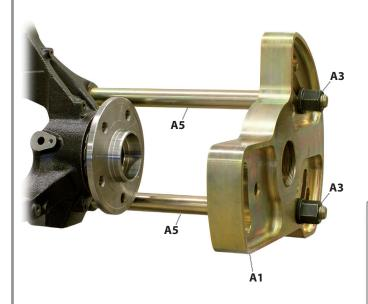
**3.** Place the base plate [A1] in the correct position on the support rods [A5] according to the **hole distance** of the base strip [E..] as shown.
