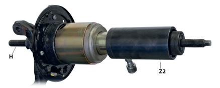
2. Prepare the hydraulic cylinder [Z2] accordingly as shown and insert it with the *PULL SIDE* on the wheel bearing.
