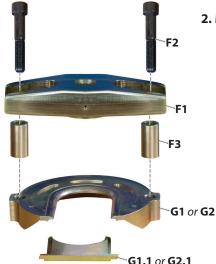
**2.** Mount the bridge [F..] as shown, in the correct position onto the tension / pressure plate [G..] and tighten both screws [F2] with **30Nm**.
