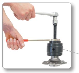
(i) If the wheel hub is to be used again, the wheel bearing inner ring must be removed first. For example, with the help of the **puller kit for bearing inner rings - KL-0042-90 K**, which is available as an *accessory*
