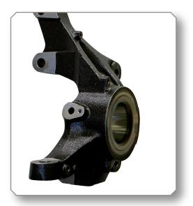
**5.** Check the correct installation position of the wheel bearing according to the manufacturer's specifications, remove the wheel bearing tool and, if necessary, insert the wheel bearing retaining ring on the steering knuckle.
