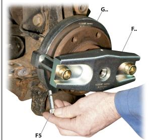
**3.** Place the bridge **[F..]** with tension/pressure plate **[G..]** in the correct position over the wheel bearing unit as shown.
