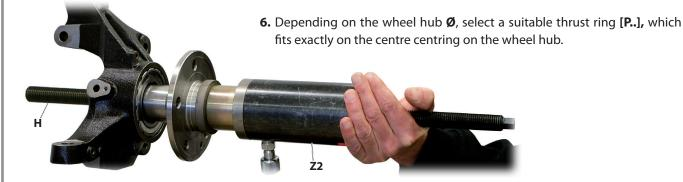
7. Prepare the hydraulic cylinder [Z2] accordingly as shown and insert it with the *PULL SIDE* on the wheel bearing.
