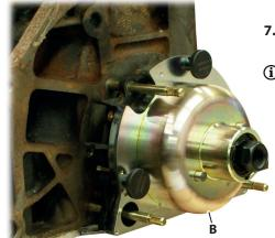
7. Place the housing [B] on the assembly tool so that both dowel pins [A4] and **both** dowel pins **[C4]** fully engage in the **four** holes on the housing **[B]**.
