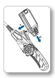
(i) The display unit [B] has a permanently installed lithium polymer battery. Charge it using the enclosed mains adapter [D] with charging cable [E1].
