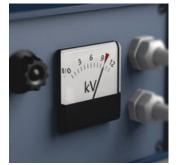
Our screwdrivers are tested for dielectric strength under a 10,000 volt load to make sure that their most important property, their insulation, has been exhaustively tested. Each individual Wera VDE screwdriver is subjected to this test to guarantee safe working up to 1,000 volts.
