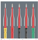
Reduced blade diameter with integrated protective insulation, allows sunken screws and spring elements to be accessed and actuated, individually tested as per IEC 60900.
