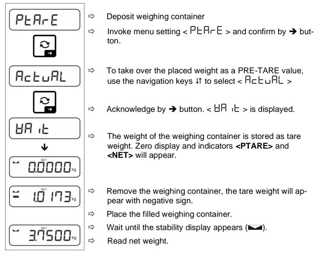
The entered tare weight remains valid until a new tare weight is input. To delete press the TARE key or confirm the menu setting  $< \Box L \Box \Box = 0$  using the  $\rightarrow$  button.
