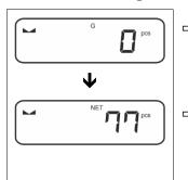
$\Rightarrow$  If necessary, put on and tare the weighing container.
