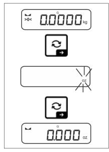
The unit for quick selection can be determined when the  $rac{2}$ -button is shortly pressed for the first time.
