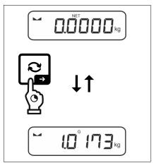
⇒ Keep the the button pressed until the display shows the gross weight value.
