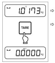
Put weighing container on the weighing plate.
