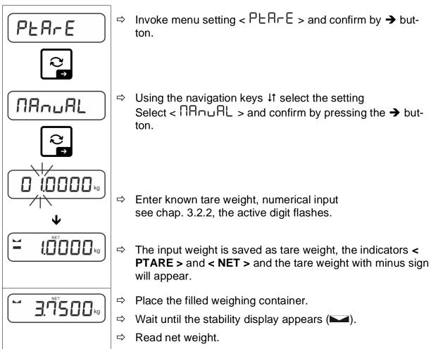
The entered tare weight remains valid until a new tare weight is input. To delete enter the zero value or confirm the menu setting  $< \Box L \Box \Box = 0$  using the  $\rightarrow$  button.
