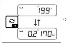
Using  $\overrightarrow{\sim}$  button, it is possible to switch over between the enabled unit 1 and unit 2.
