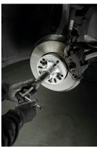
The hydraulic hub puller of series 229 is used for pulling all 4- and 5hole hubs of almost all types of passenger cars in Automotive and Industry. The flange is designed with slots of different pitches for accepting standard screws.
