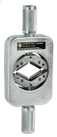
The thread restorers of the W-714 series are used to repair damaged threads and similar parts in craft, industry, and workshop. The thread restorers are capable of reliably restoring threads even on special parts, which would otherwise be significantly more expensive to purchase new.
