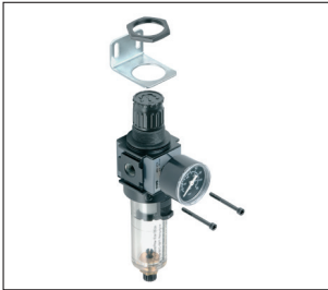
Module attachment by fixing bracket (for regulator) or direct mounting (2 screws) for all units.
